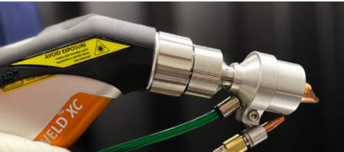
Gas Lens Nozzle Ideal for materials sensitive to oxygen, moisture, or other atmospheric gases, this nozzle features a precision laser-drilled diffuser in a showerhead configuration.
