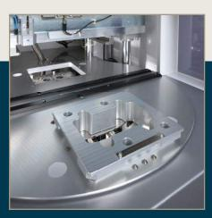
The calibration tools specifically optimized for the EvoWeld enable rapid checking of the essential process parameters with minimum time expenditure. Our EvoLaP process software easily guides the machine setter through the relevant procedure, automatically
